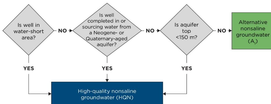
**Figure 1. Decision tree for determining if nonsaline groundwater should be treated as “high-quality” or “alternative”**
